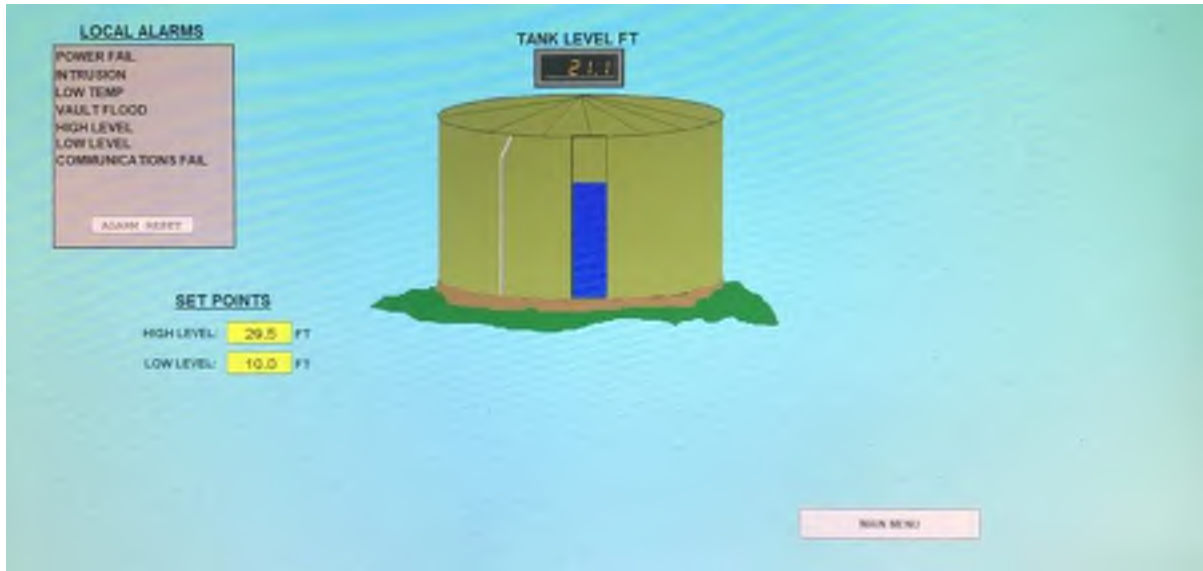
FIGURE 1-2 Prospect Street Water Storage Tank SCADA GUI
